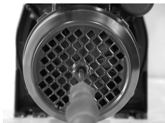
In order to avoid mechanical seal blocking, turn the shaft through the motor fan before starting up or after extended unuse!
