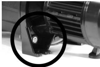
Regularly check the waterproofness! (A leak through a mechanical seal can cause important damages!)
