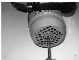
In order to avoid mechanical seal blocking, turn the shaft through the motor fan before starting up or after extended unuse!
