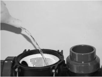
Prime the pump (if not risk of dry running). WARNING! RANTY LOSS!!!
